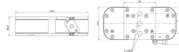
The normal position of the indicator is as shown position "N", position "E" on request only.
