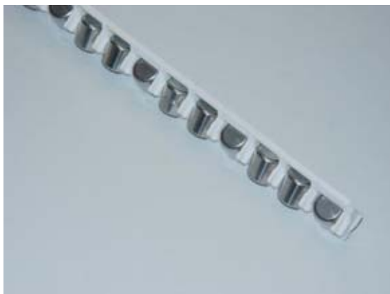
Linear cross roller cage Arrangement of rollers 2:1 (2 support rollers / 1 holding roller)
