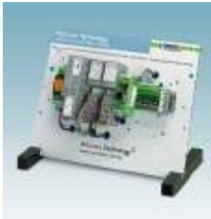
Starter kit for automation with PLCnext Control
