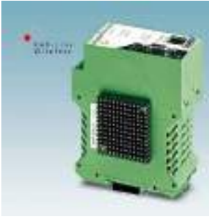
900 MHz – Wireless transceiver with Trusted Wireless, for Ethernet
