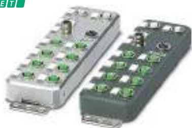
8 digital inputs and 8 digital outputs
