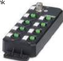
1 IO-Link A port 8/16 digital inputs
