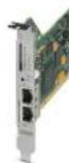
Router with firewall and VPN for PCIe
