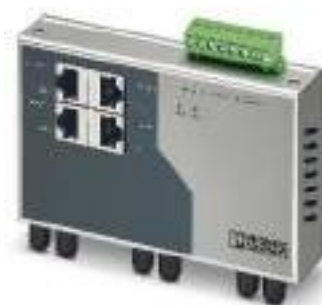
4 RJ45 ports and 3 FO ports
