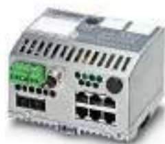
6 RJ45 ports and 2 SFP ports
