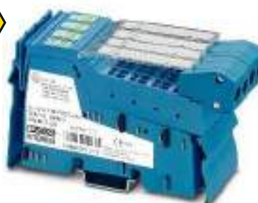
4 selectable temperature inputs, RTD or TC
