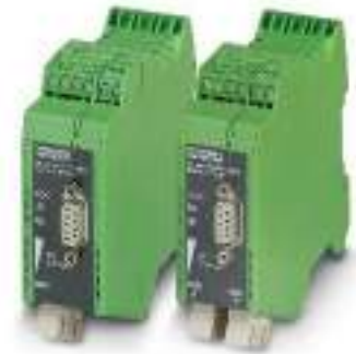
PROFIBUS fiberglass (multimode and single mode)
