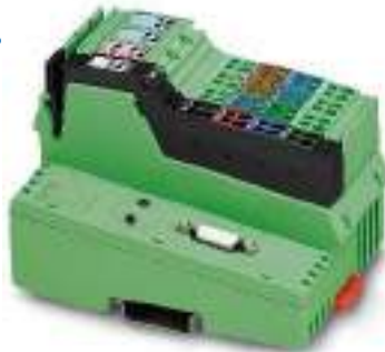
D-SUB connection, 8 digital inputs and 4 digital outputs
