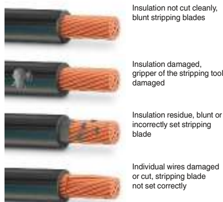
Cable stripped incorrectly in accordance with DIN IEC 60352-2
