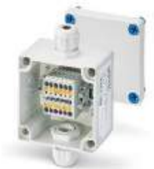
Terminal box with 6 2.5 mm² terminal blocks with Push-in connection technology
