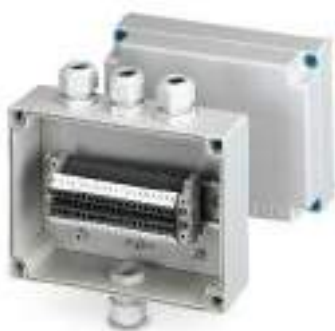
Terminal box with 20 2.5 mm 2 terminal blocks and screw connection technology
