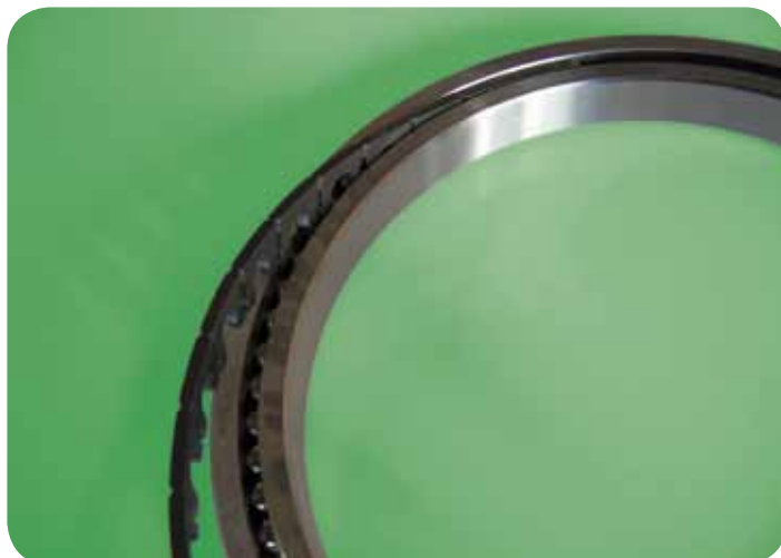
Integration of the snap-over separator strip
