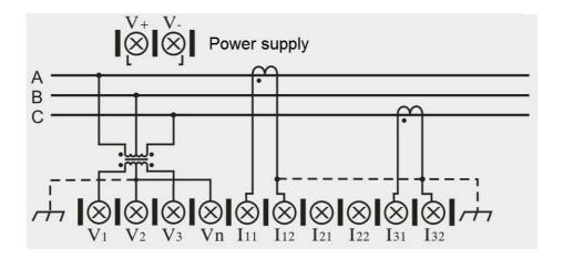
Figure 5-5 Wiring Diagram of 3-phase-3-wire
