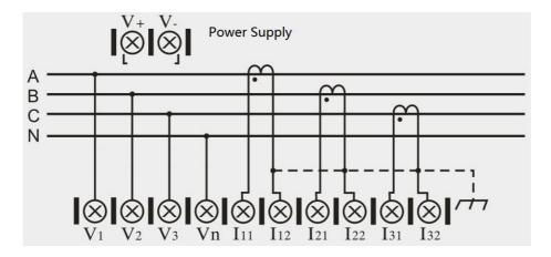
Figure 5-3 Wiring Diagram of 3-phase-4-wire (W/O PT)
