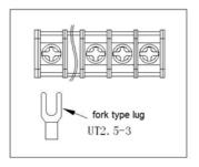
Figure 5-2 Connection Diagram of Main Terminal
