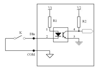
Figure 3-2 Circuit Diagram of Binary Input Interface
