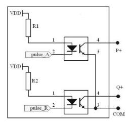
Figure 3-1 Circuit Diagram of Power Pulse Output Interface
