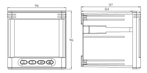
Figure 5-1 Overall Dimension of Instrument
