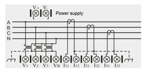
Figure 5-4 Wiring Diagram of 3-phase-4-wire (With PT)
