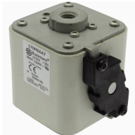
Fuse-link, high speed, 550 A, AC 2500 V, size 3, 86 x 95 x 166 mm, aR, IEC, single indicator
