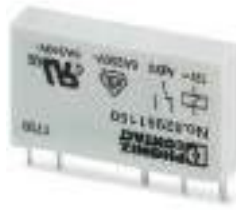
Relay with one changeover contact, max. 6 A
