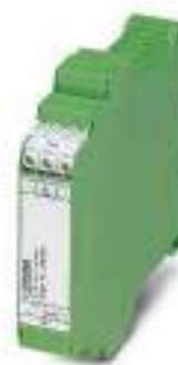
Voltage measuring module, 0...1,500 V DC
