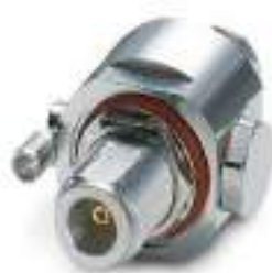
For GSM systems (0 - 3 GHz), grounded shield, connection: type N
