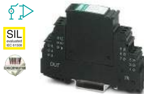
4-conductor with common reference potential, connection 9/10 grounded via gas-filled surge arrester, e.g., for binary signals
