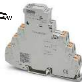
Transceiver module for remote signaling of TTC-6...-I products
