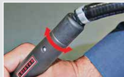
Swiveling air hose for easy working.
