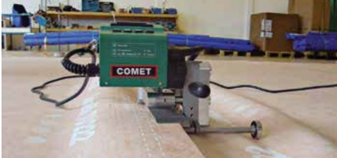
Hands-free welding due to integrated guiding plates.
